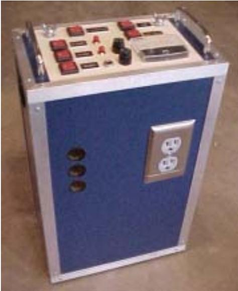
To free my telescope from its power connection to my vehicle when observing at remote sites, I made a power supply box to furnish 18VDC for the LX200 telescope, as well as 12VDC and 120VAC for accessories. The box provides all the power I need without having to cobble together anything in the field.
